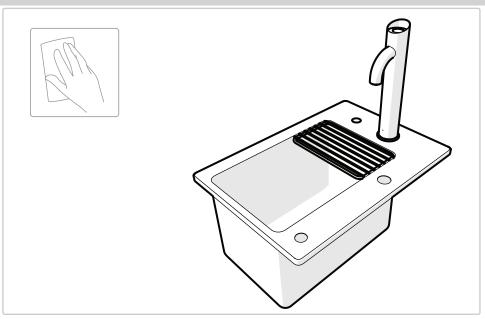
The exterior of this font may be cleaned with a damp cloth and a light detergent. Do not use abrasive cloths or creams, as this will spoil the finish of the font. Do not use a water jet or spray. Beware of accidentally operating the font when cleaning the top of the font.
