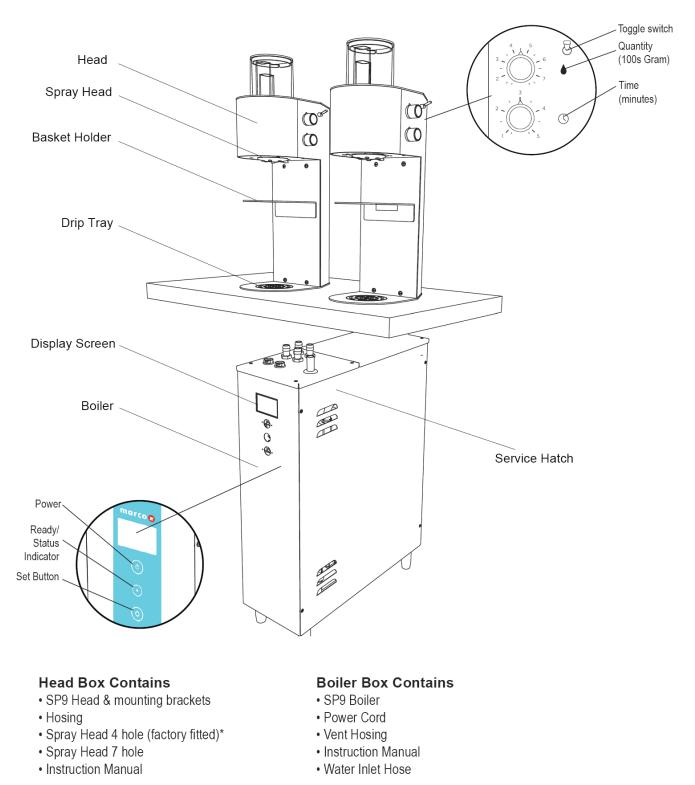
\* Note: Alternate spray head not suitable for cup-by-cup swapping. Preferred sprayhead should be selected at install prior to calibration.
