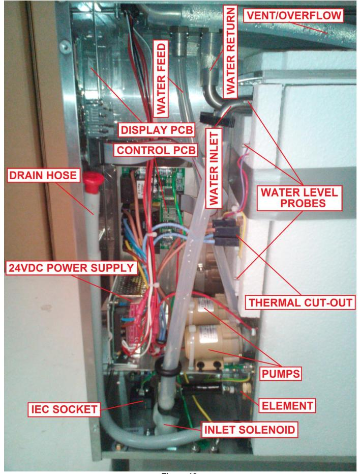
Figure 13. Main Control Board Connections
