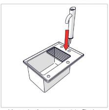
Mount the font on the sink. Placing the threaded bar, hose and wiring through the hole.
