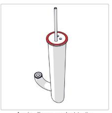
Apply silicone sealant to the bottom of the font in the area marked in red.
