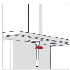
Firmly tighten the mounting plate to the base of the sink, making sure not to catch the wiring.
