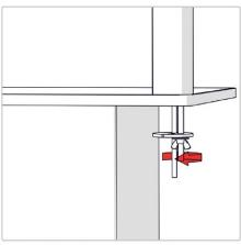
Tighten the wing nut up while threading the wiring and tube through the mounting plate.
