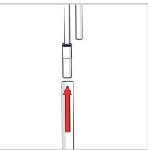
Attach the silicone tube supplied to the fitting on the hose and cut to lenght. Please ensure the hose is straight and free of any bends.
