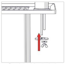
Place the mounting plate back through the threaded bar,hose and wiring. Screw the wing nut back on with the washer.
