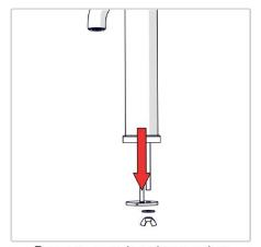
Remove mounting plate, washer and wing nut from the bottom.
