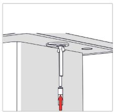
Place the fitting supplied to the hose. **PUSHING FIRMLY**
