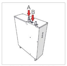
Attach the silicone tube to the water outlet (A). Connect the wiring from the font to the four way connector (B).
